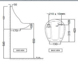
ALL DIMENSIONS ARE IN MM. (TOLERANCE ± 5 MM)
